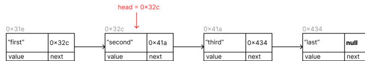
Figure 4.5: The linked list is an abstract data structure which acts as a fundamental conceptual entity in computer science. It is here represented as a graph, and implementations can be seen in 57 and 59.
